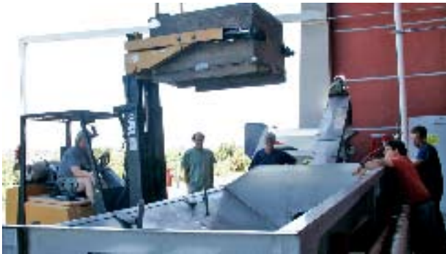
Delta Destemmer Crusher (in back), Receiving Hopper, Conveyor, Michael Blaylock, Winemaker Operating Forklift
